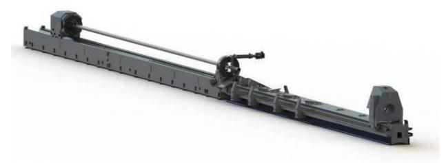
In the first phase of cutting process, M1 drives the tube through M2 and then to the cutting area, where the trimming of the first end is performed. The CN controlled manipulators, positioned in the loading area, assist the mandrels (chucks) with the support of the tube. The correct alignment of the tube is granted.
