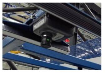
Through a software tool and directly from the HMI of the machine, the operator can easily import the reference template. The detection of the welding seam depends on the environmental light and on the tube surface condition. Due to the optic principle, this system works correctly if the welding seam is well visible by human eye from the external and the surface is free of scratches.
