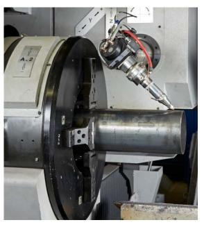
Through a sensor, it is possible to keep the exact focusing distance from the surface to cut. Furthermore, thanks to this sensor, any eventual collisions between the head and scraps or other parts are avoided.
