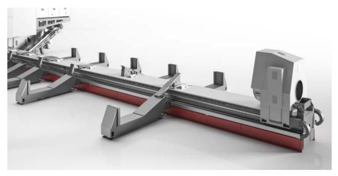
The first and the third mandrel (chuck) (M1 and M3) are expected to clamp the tube ends.
